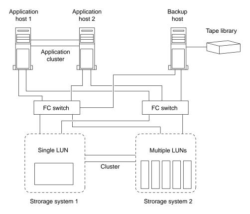
Volumes on a host can consist of a single LUN mapped from the storage system or multiple LUNs using a volume manager, such as VxVM on HP-UX systems.
